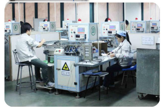
automatic resin injection machine, automatic internal resistance detection machine for A type
